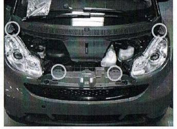
Open the door and remove the antenna. Remove the two clips, one from the fender and one from the antenna cover and close the door.
