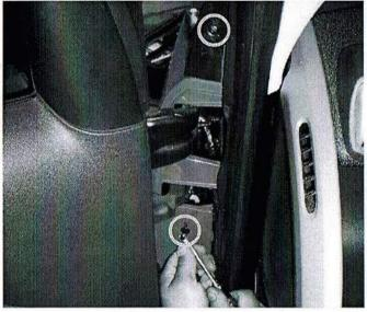
Remove the antenna cover and the two screws behind the antenna cover.
