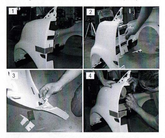
13) Close the door and replace the fender. Use the "L" bracket you installed earlier to secure the inner fender as shown.
